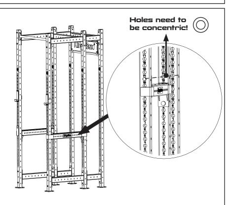
When attaching the safety catchers make sure that the holes of the uprights are concentric - aligned!
